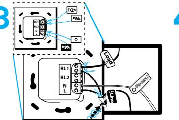
Insert the Neutral wire into the screw terminal labeled with N. Insert the Line into the screw terminal L. Insert the Line and the Load into the screw terminals of RLI. If you have multiple gangs repeat the instructions. If you have a ground wire, place it into the wall box.
