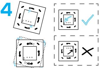
try to allow as much space for the switch as possible. Insert the iotty Light Switch in the wall box screws.
