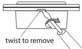
**Remove the glass panel** of a touch remote switch: Using a small flat screwdriver remove the front cover by placing the screw driver in the location notch on the bottom part of the cover and twist to unclip the cover.
