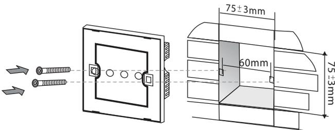
**Fix screws:** Use the screws supplied to attach switch to backbox using a flat head screwdriver
