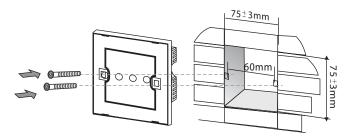
Fix screws: Use the screws supplied to attach switch to backbox using a flat head screwdriver
